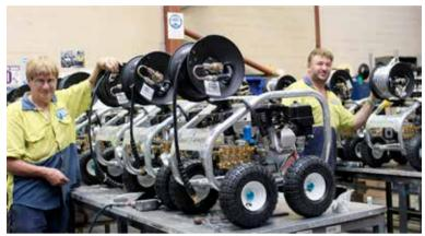
Aussie 'Pocket Rockets', with integrated hose reels, roll off the Castle Hill works production line.
